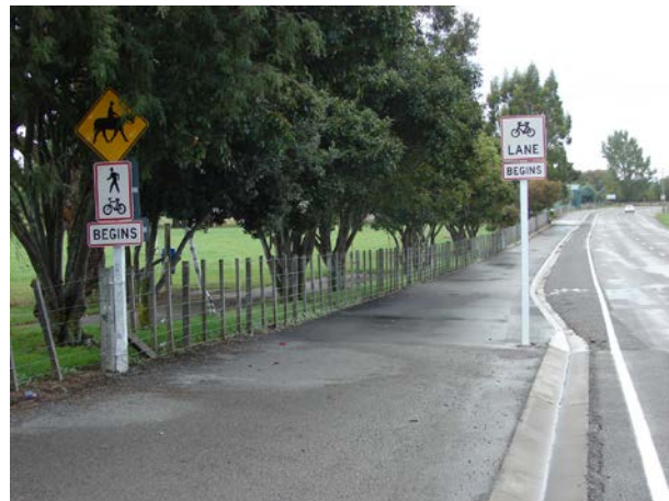
These improvements to Colombo Road, near Lakeview School, provided a shared path for school cyclists, and also on-road cycle lanes for the more confident cycle tourists who will also use this route
